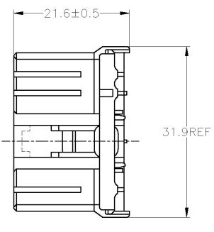
⚠ MUST BE KEPT BETWEEN -A- AND 2 ▲ TO BE MATED WITH THE CAP HOUSING SMOOTHLY
