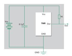
Note: It is strongly recommended that an external bypass capacitor be connected in-close-proximity to the device between the supply and ground pins to reduce noise. The recommended value for the external bypass capacitor is 0.1µF.
