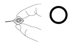
Don't pull fan with lead wires.
