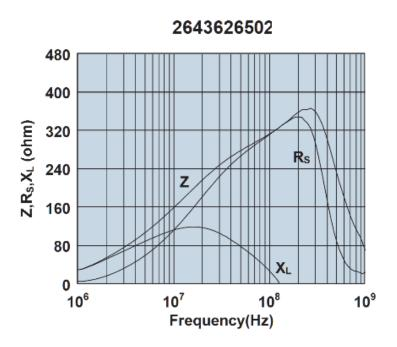
Impedance, reactance, and resistance vs. frequency.
