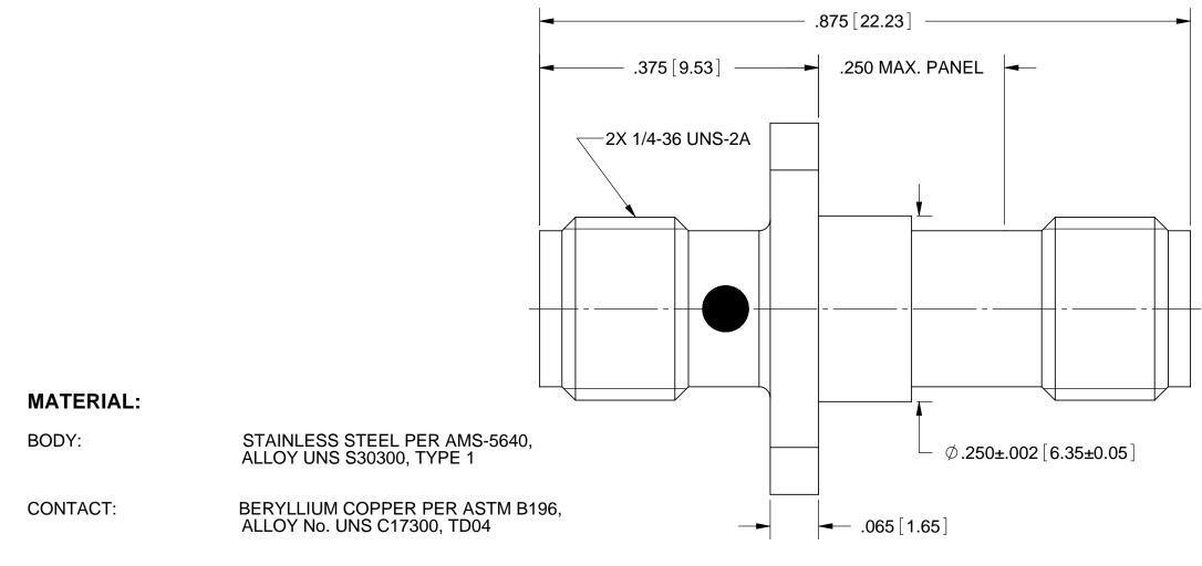
**INSULATOR:** PTFE PER ASTM D1710, TYPE I, GRADE 1, CLASS B
