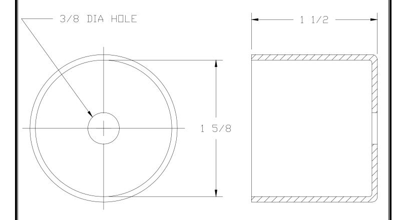
Recommended especially for 110Vac & 250Vac models, or any other classic ('SC') Sonalert<sup>®</sup> model where terminal insulation is desired.
