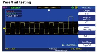
Generate user-defined pass/fail limits to quickly identify go/no go test results.
