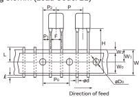
Outside Crimp Taping Lead Spacing 2.5mm (Lead Code: S1)
