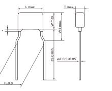
\* Coating extension does not exceed the end of the lead bend Lead Wire: Solder Coated CP Wire
