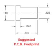
Standard Tolerances: Lengths: ±.006 Diameters: ±.002 Angles: ±2"
