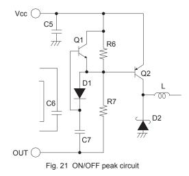
Since the PNP Tr is generally slow in switching, in terms of the sat characteristics , the ON/OFF peak circuit is used as an acceleration circuit. The D1 and the C7 generate an ON peak current, while the Q1 and the C7 forms an OFF peak circuit.Set pull-up resistance to 510  $\Omega$  as a guide at VCC=12 V. It is recommended to set this resistance in the range of 100 kΩ to 10 kΩ. In order to make adjustment of the R6 and R7, however, pay attention of the points listed in table below.
