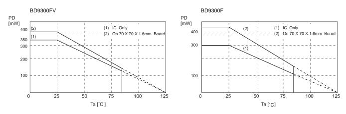
Fig. 29 Thermal derating characteristics
