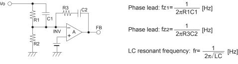
Fig. 25 Typical circuit after secondary compensation circuit
