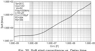
Fig. 20 Soft start capacitance vs. Delay time
