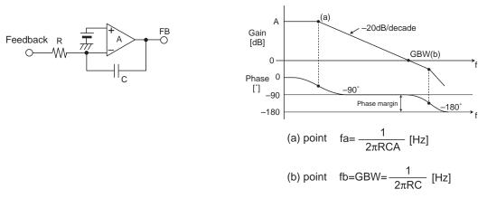
Fig. 22 Typical integrator characteristics
