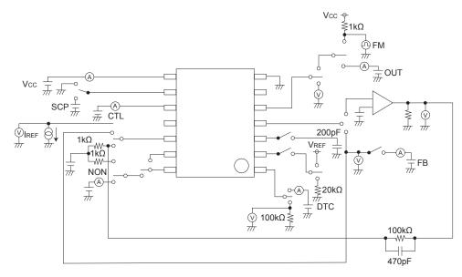
Fig. 1 Typical measurement circuit
