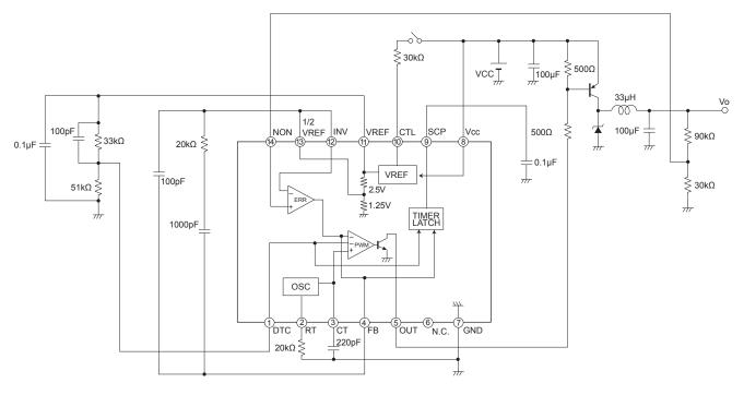
Fig. 12 Typical application circuit
