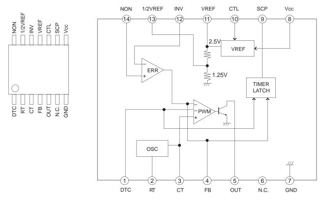
Fig. 11 Pin assignment / Block diagram
