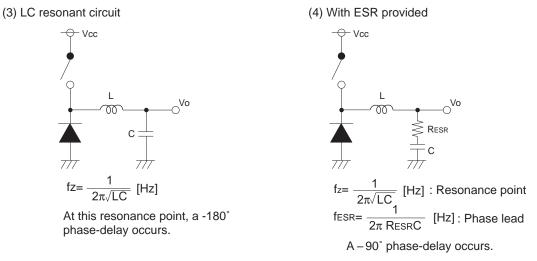
\* Same for the phase compensation of inverting and step-up voltages
