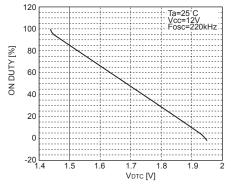
Fig. 19 DTC voltage vs. Maximum duty
