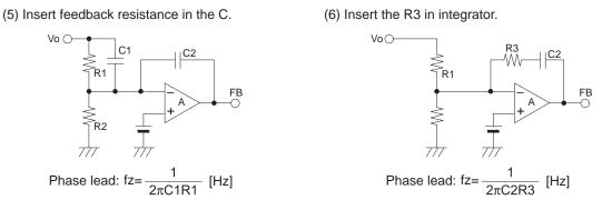
Fig. 24 Typical phase compensation circuit
