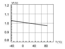
Fig. 3 Forward Voltage vs. Temperature
