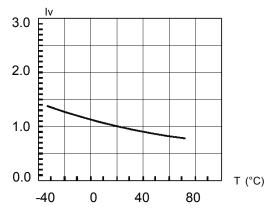
Fig. 4 Relative Luminous Intensity vs. Temperature
