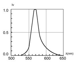
Fig. 1 Relative Luminous Intensity vs. Wavelength
