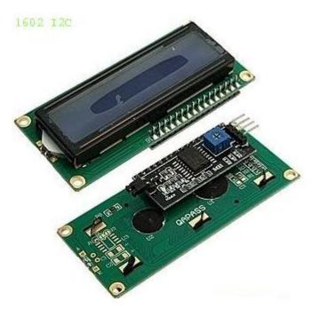
Arduino IIC LCD1602 / I2C interface adapter plate with LCD screen
