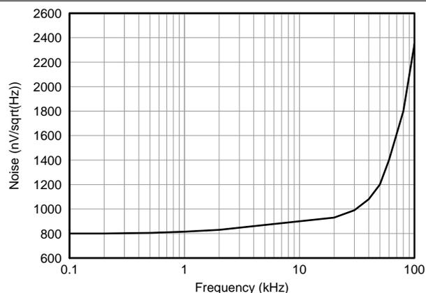
**Figure 38. Output Noise Density of the AMC1100**
