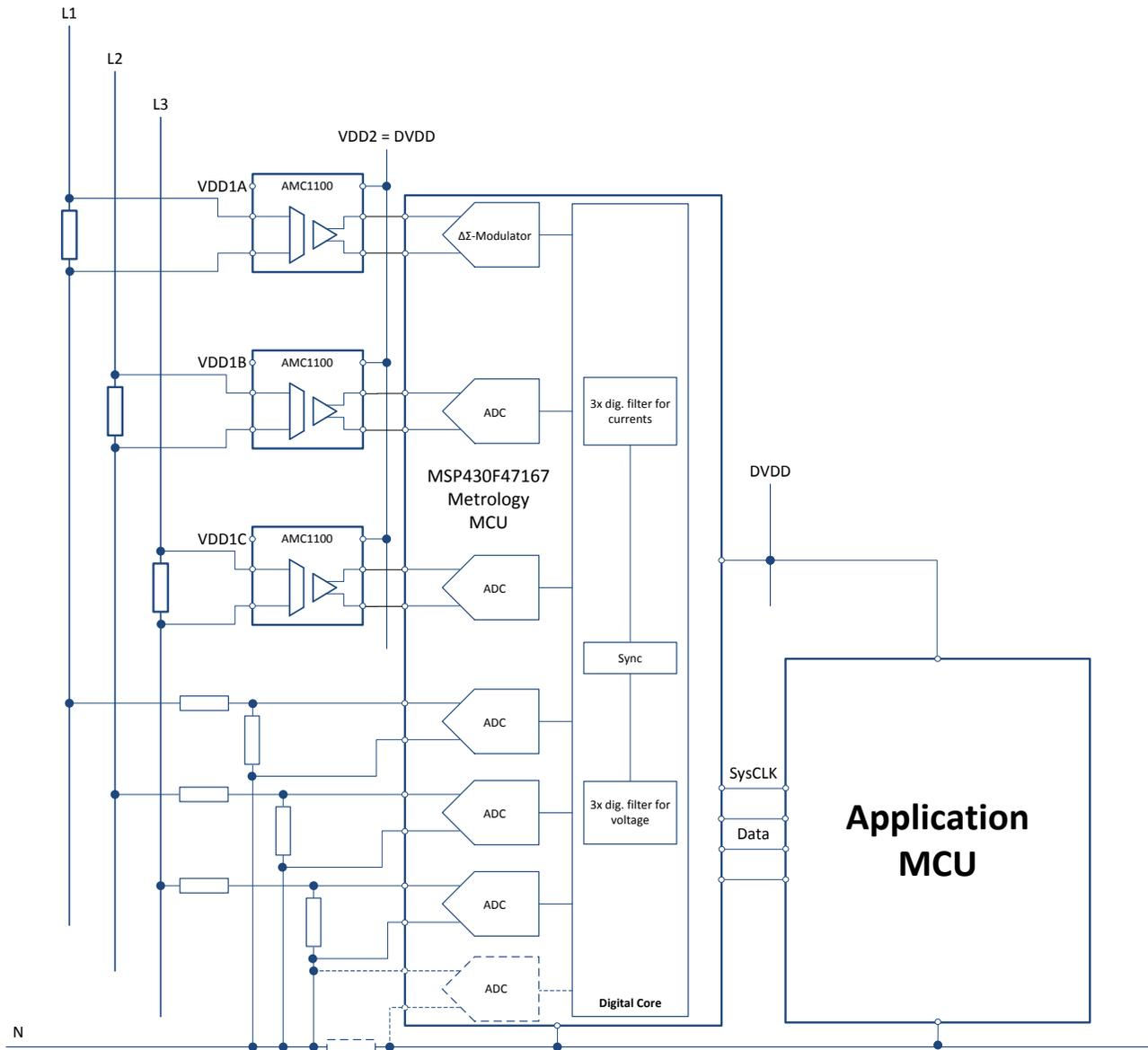
Figure 36. The AMC1100 in an E-Meter Application
