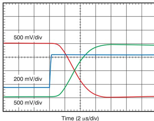
Figure 35. Typical Step Response of the AMC1100
