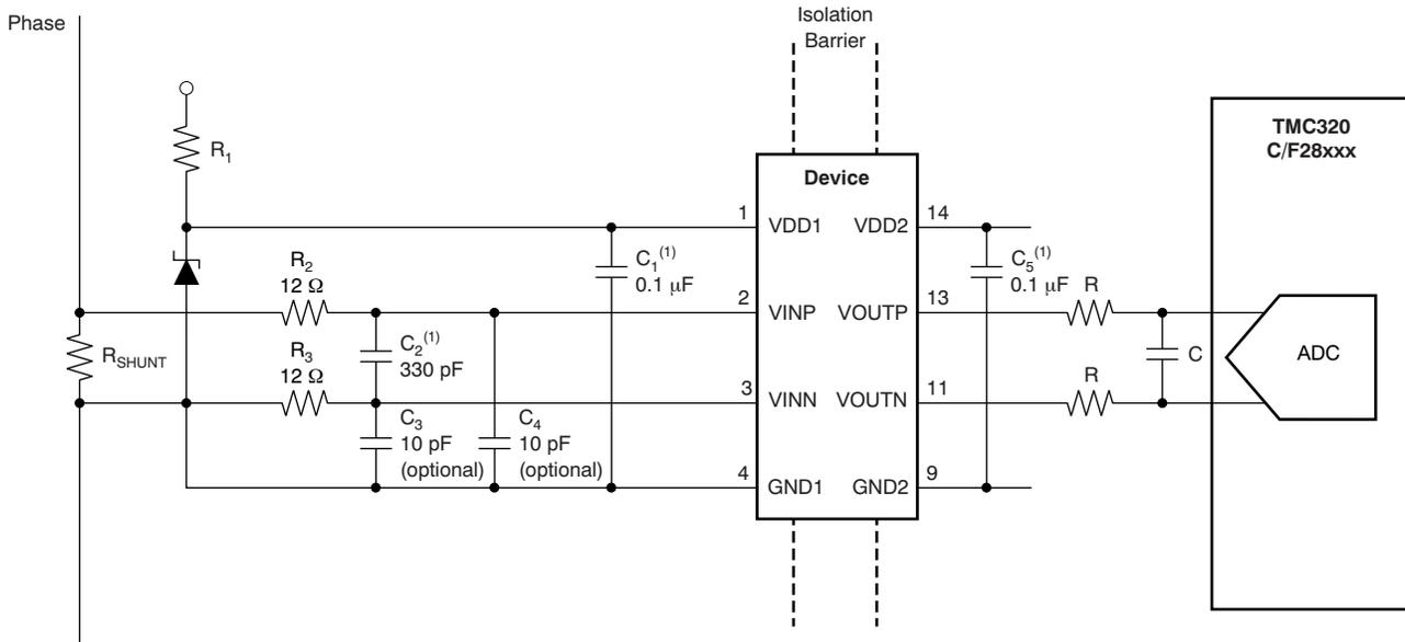
Figure 34. Shunt-Based Current Sensing with the AMC1100
