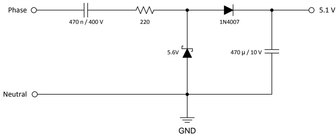
**Figure 37. Cap-Drop High-Side Power Supply for the AMC1100**
