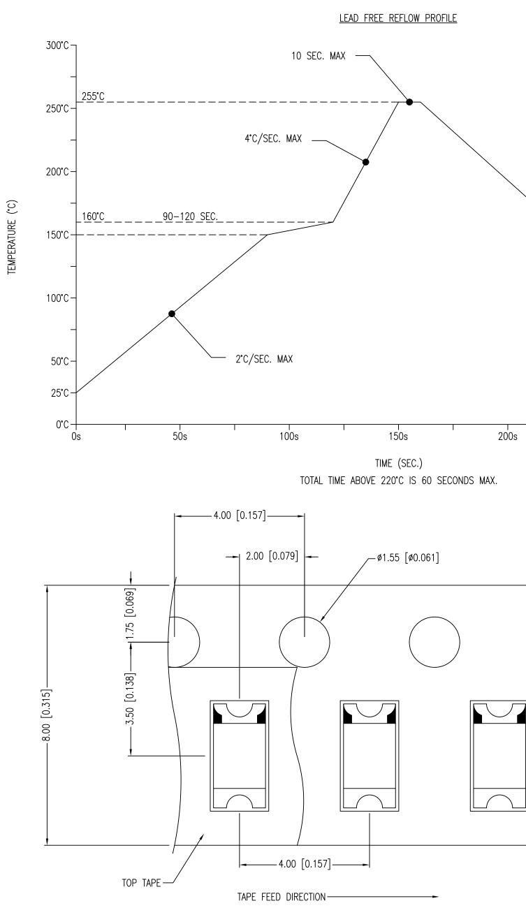
\*UNLESS OTHERWISE SPECIFIED TOLERANCES PER DECIMAL PRECISION ARE:  $X = \pm 1$  (±0.039),  $X = \pm 0.5$  (±0.020),  $X = \pm 0.25$  (±0.010),  $X = \pm 0.127$  (±0.005). LEAD SIZE=±0.05 (±0.002), LEAD SIZE=\pm0.05 (±0.002), LEAD SIZE=\pm0.05 (±0.002), LEAD SIZE=\pm0.05 (±0.002), LEAD SIZE=\pm0.05 (
