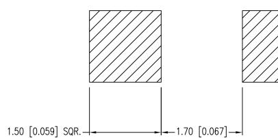
\*UNLESS OTHERWISE SPECIFIED TOLERANCES PER DECIMAL PRECISION ARE: X=±1 (±0.039), X.X=±0.5 (±0.020), X.XX=±0.127 (±0.005). LEAD SIZE=±0.05 (±0.002), LEAD LENGTH=±0.75 (±0.030). MIN=  $^{+DECIMAL}_{-0.00}$  MAX.=  $^{+0.00}_{-DECIMAL}$  PRECISION MAX.=  $^{+0.00}_{-$
