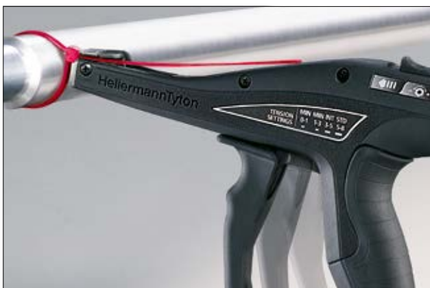
1. Tension: Tie is tensioned as usual.
