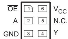
DRY package 6-pin SON (Transparent Top View)
