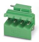
PCB header, nominal cross section: 2.5 mm², color: green, nominal current: 12 A, rated voltage (III/2): 320 V, contact surface: Tin, type of contact: Male connector, Number of potentials: 4, Number of rows: 1, Number of positions per row: 4, number of connections: 4, product range: MSTBO 2,5/..-G1L, pitch: 5 mm, mounting: Wave soldering, pin layout: Linear pinning, solder pin [P]: 3.5 mm, Locking: without, type of packaging: packed in cardboard, Product with pin output on left side
