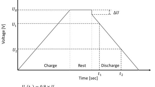
$U_1(t_1) = 0.8 \times U_R$  $U_2(t_2) = 0.4 \times U_R$
