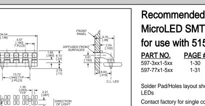
NOTE: designed for post-reflow PC board insertion.
