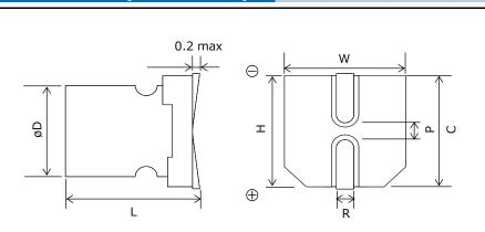
Unit : mm Size P±0.2 W±0.2 øD±0.5 H±0.2 C±0.2 R code 5.0 5.9 5.3 5.3 6.0 0.6 to 0.8 1.4 В6 6.3 5.9 0.6 to 0.8 6.6 6.6 7.3 2.1 C6 E7 8.0 6.9 8.3 8.3 9.0 0.6 to 0.8 3.2 9.0 E12 8.0 11.9 8.3 8.3 0.8 to 1.1 3.2 F10 10.0 10.0\*1 10.3 10.3 11.0 0.8 to 1.1 4.6 10.0 12.6 10.3 10.3 0.8 to 1.1 4.6 F12 11.0 \*1:±0.5
