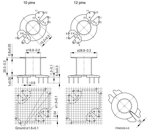
Hole arrangement View in mounting direction
