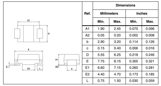
Figure 17. SMC footprint dimensions in Figure 18. Marking layout<sup>(1)</sup> mm (inches)
