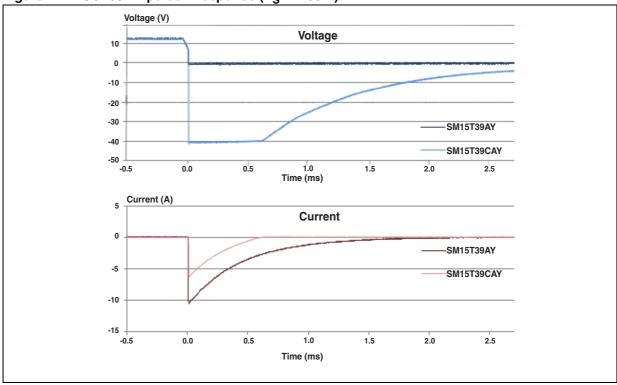
Figure 13. ISO7637-2 pulse 2 response ( $V_S = 50 \text{ V}$ )
