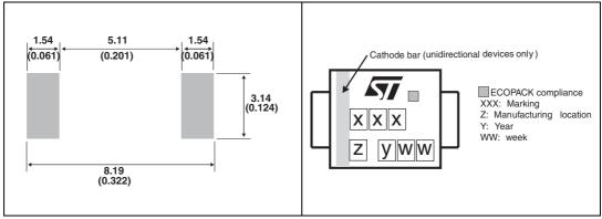
1. Marking layout can vary according to assembly location.
