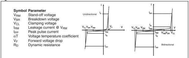
Figure 2. Pulse definition for electrical characteristics
