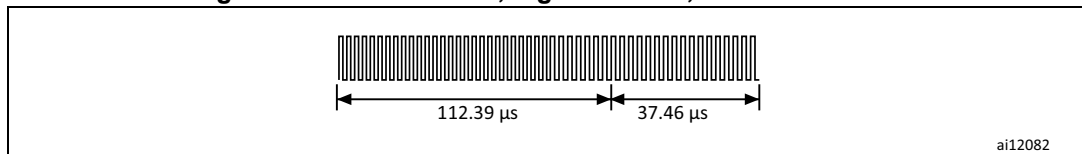
Figure 39. Start of frame, high data rate, two subcarriers
