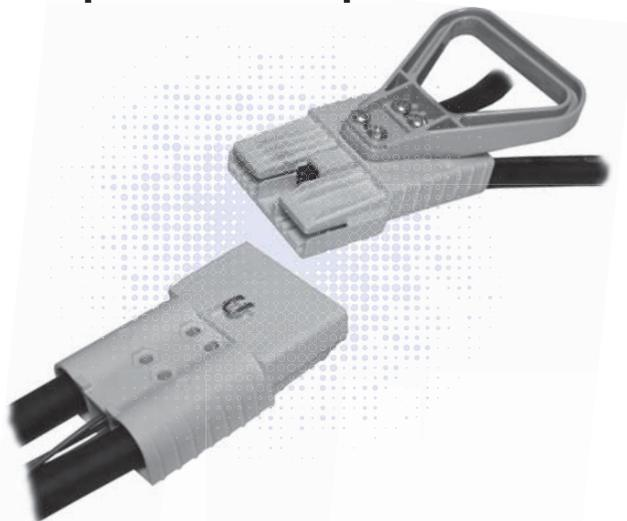
SBX® and SBE® connectors can integrate up to 8 auxiliary power / signal contacts along with the two primary power circuits. Sequencing within auxiliary positions is possible using the 4 pin lengths available in the 1x4 auxiliary connector. The SBE® touch safety rating is equivalent to that of the SBS® connector line.
