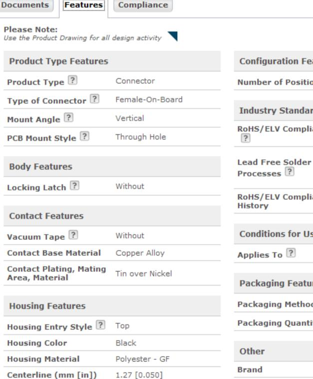
**Configuration Features** Number of Positions ? 16 **Industry Standards** RoHS/ELV Compliance RoHS compliant, ELV compliant Wave solder capable to 240°C, Wave solder capable to 260°C, Wave solder capable to 265°C RoHS/ELV Compliance Always was RoHS compliant **Conditions for Usage** Printed Circuit Board
