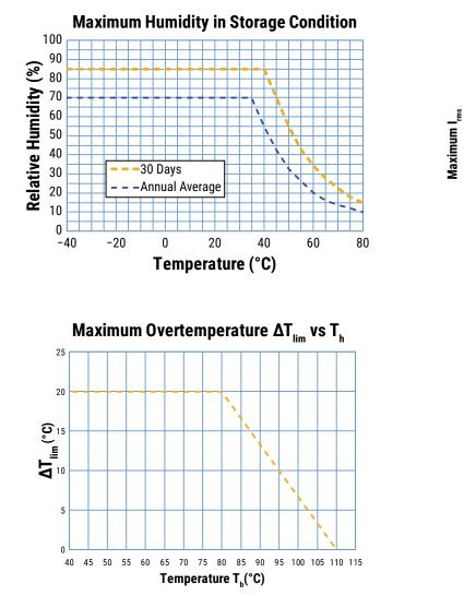
$T_h$  is the maximum ambient temperature surrounding the capacitor or hottest contact point (e.g. tracks), whichever is higher, in the worst operation conditions in °C.
