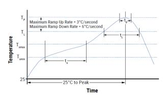
Note : All temperatures refer to the center of the package, measured on the capacitor body surface that is facing up during assembly reflow.
