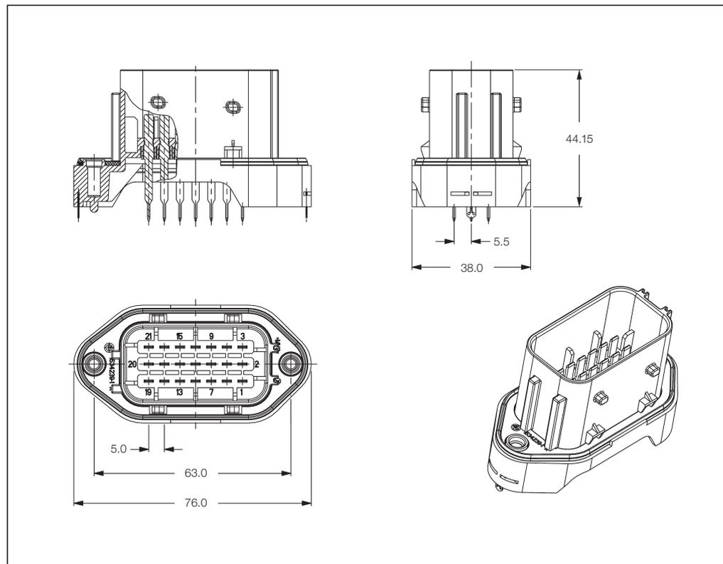
Sealed Tab Housings – Printed Circuit Board Headers
