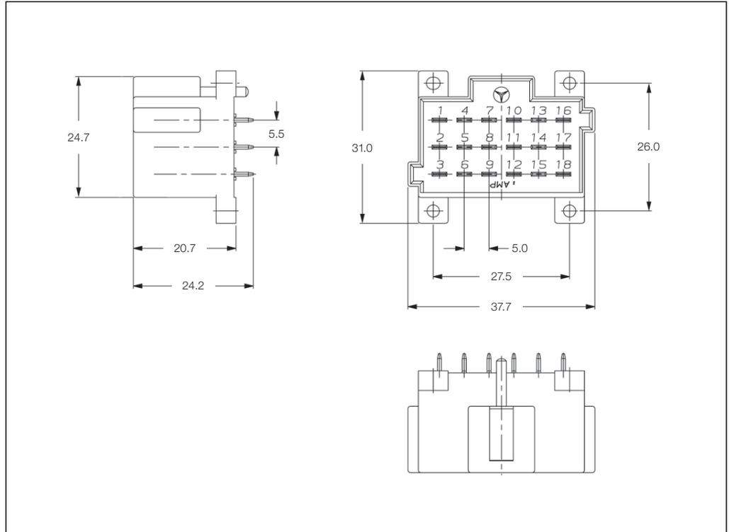
Unsealed 2.8 mm Housings – Printed Circuit Board Headers
