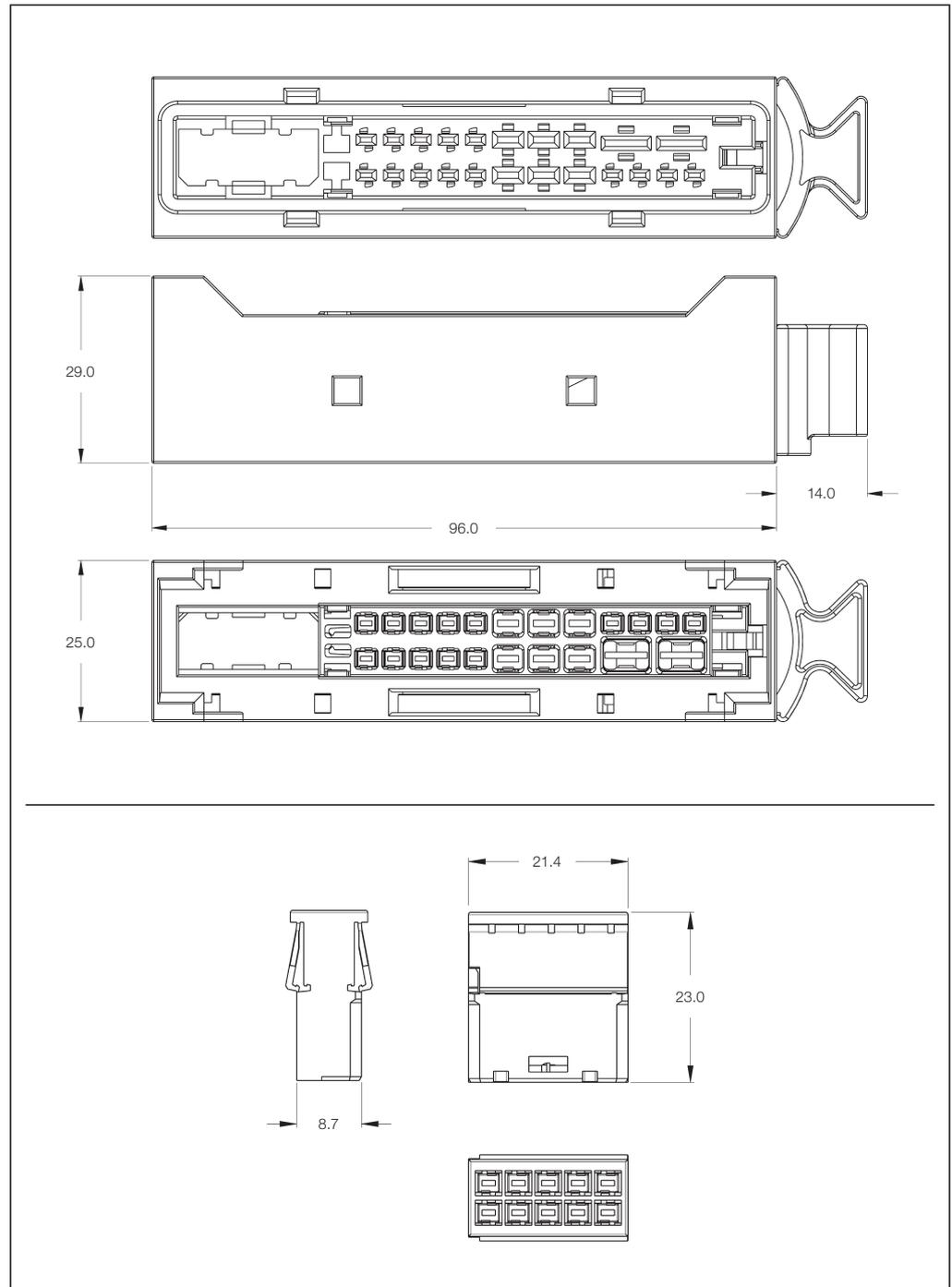
**Receptacle Housings with 22 Pos. and 10 Pos. AMP MCP**
