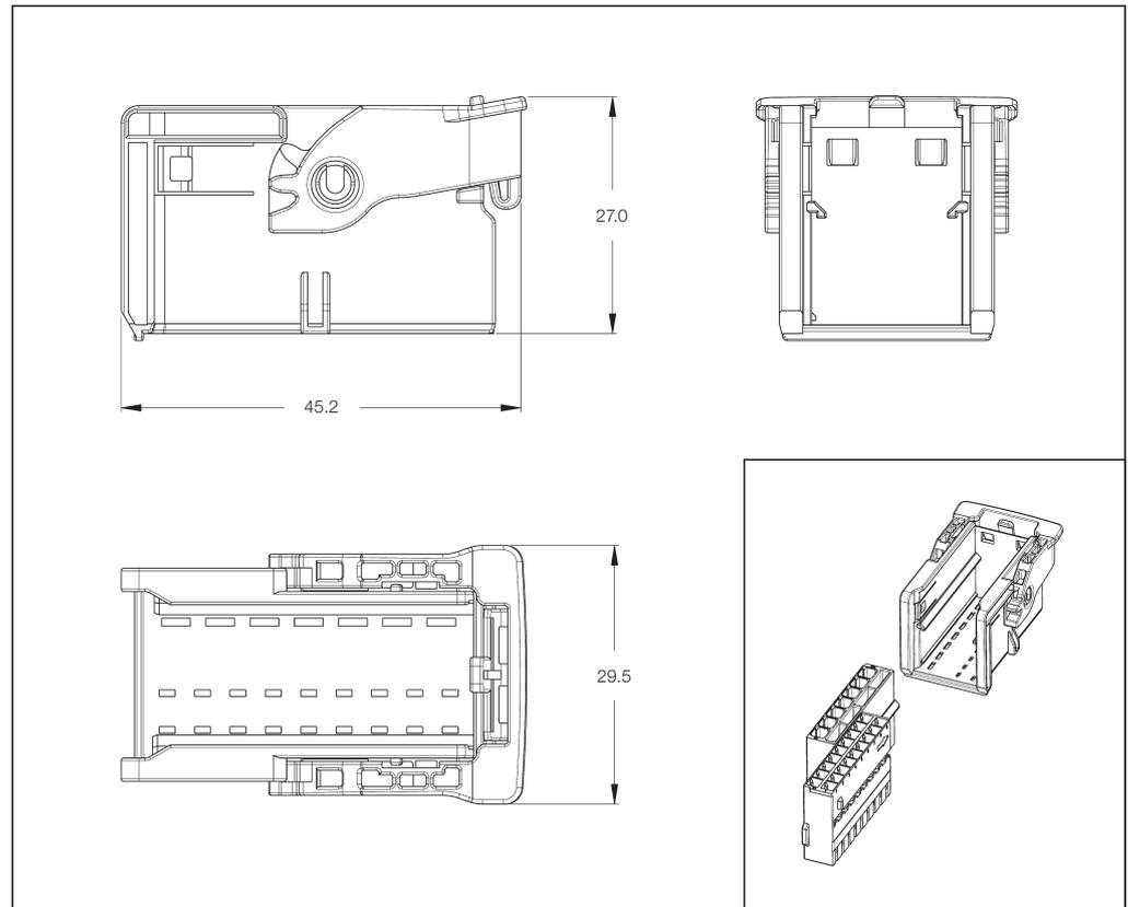
Unsealed (Carrier) Housings for AMP MCP 1.5K and AMP MCP 2.8 Receptacle Inserts
