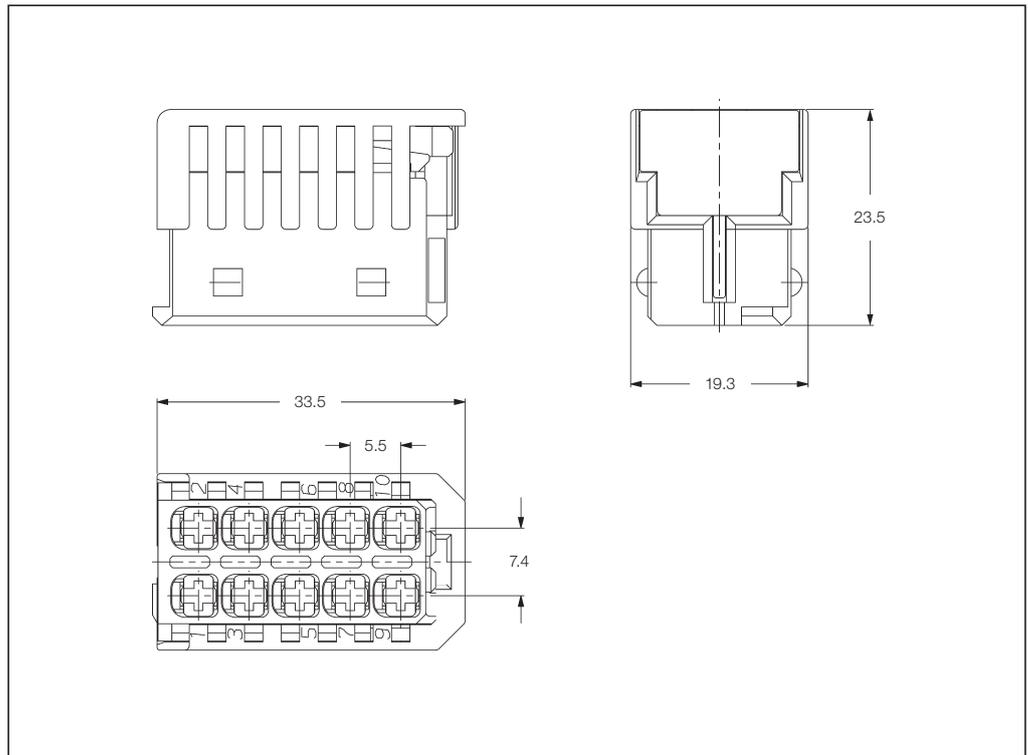
**AMP MCP 2.8 Receptacle Housings with Secondary Locking**
