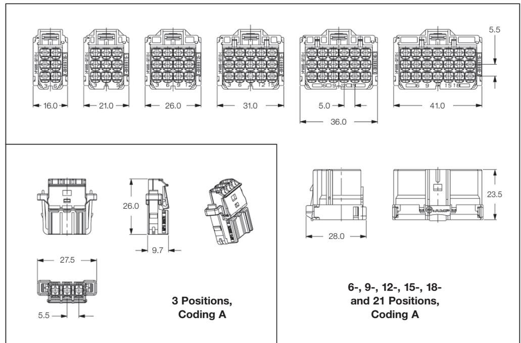
**AMP MCP 2.8 Receptacle Housings with Secondary Locking**
