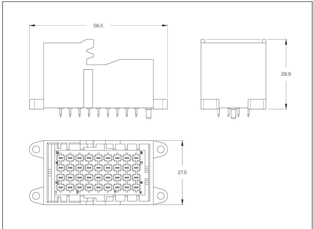
Unsealed 1.5 mm Housings – Printed Circuit Board Headers
