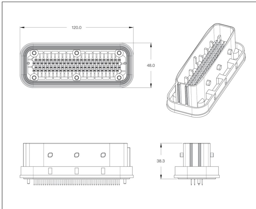
Sealed Tab Housings – Printed Circuit Board Headers
