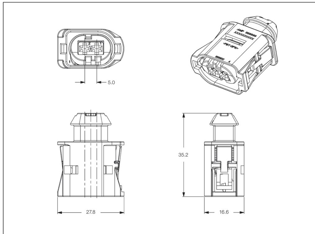
**Sealed Receptacle Housings for AMP MCP 2.8 and Sensor Flat Contacts**
