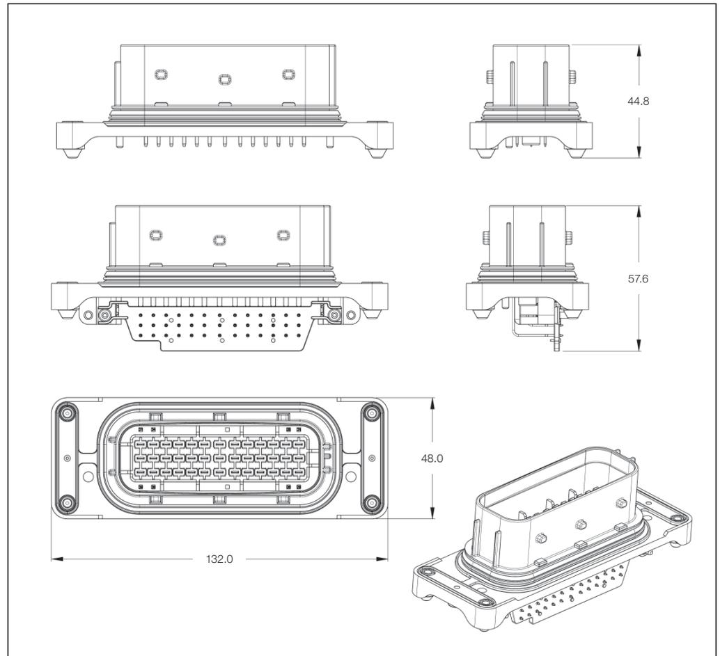
**Sealed Mixed Tab Housings – Printed Circuit Board Headers**
