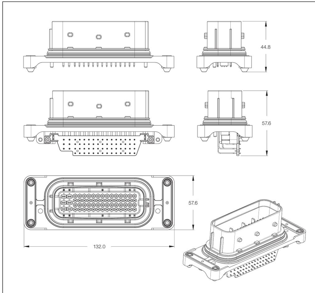
**Sealed Mixed Tab Housings – Printed Circuit Board Headers**
