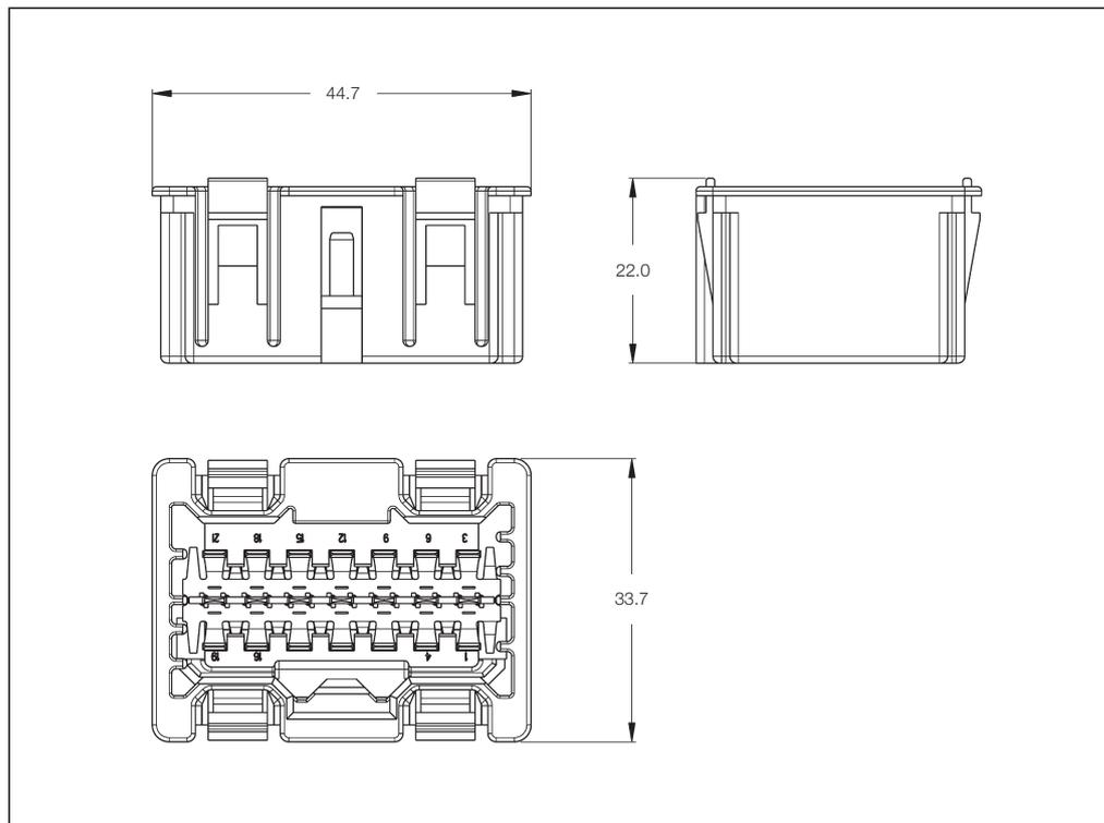
Unsealed 2.8 mm Tab Housings for Potential Distribution for Wall or Panel Mounting
