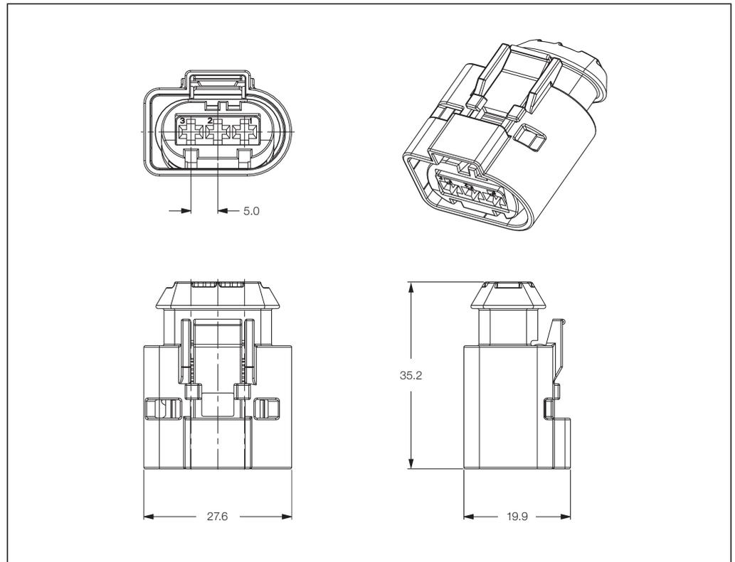
Sealed Receptacle Housings for AMP MCP 2.8 and Sensor Flat Contacts
