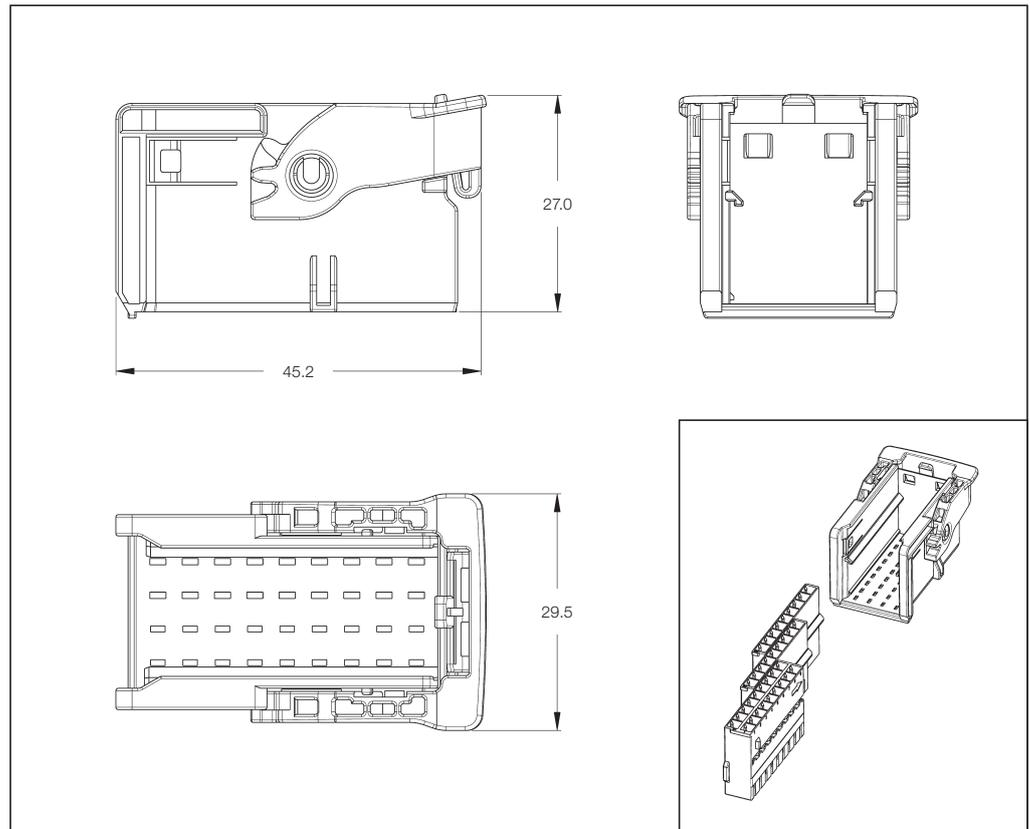
**Unsealed (Carrier) Housings for AMP MCP 1.5K Receptacle Inserts**
