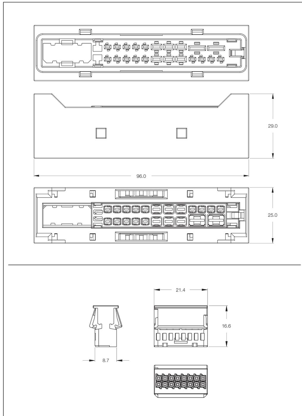
**Receptacle Housings with 22 Pos. AMP MCP + 16 Pos. MQS (Micro Quadlok)**
