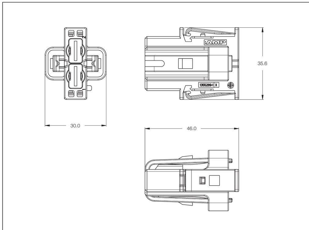
**AMP MCP 9.5 Receptacle Housings with Secondary Locking**
