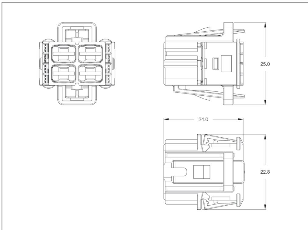
**AMP MCP 6.3 Receptacle Housings with Secondary Locking**
