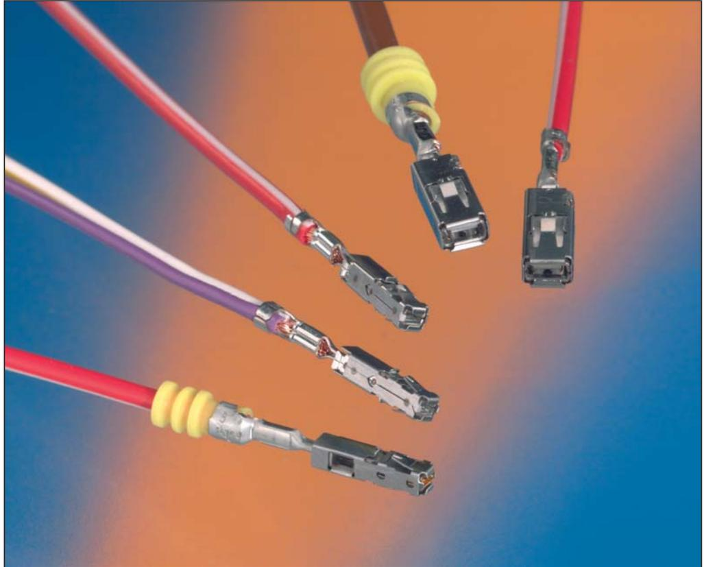
The AMP MCP Contact System is mainly used in the automotive industry. Each contact consists of a flat receptacle, which mates with a flat tab. Every contact has got a steel spring and a copper alloy body.
