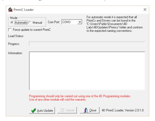
**PmmC Loader** is a GUI interface designed to download PmmC's and Drivers to 4D Systems Processors. It can automatically update existing PmmC's and Drivers present on a module, or manually change or force download to a blank processor or module, overwriting anything written in previously.
