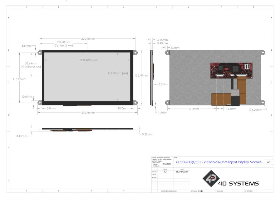
uLCD-90D Series Schematic Details (HW REV 1.5)
