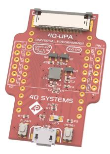
The 4D-UPA is a single module with a micro USB interface, and DIP-style pads for GPIO breakout of all the signals used on the Display interface, which is useful for development or final product use. Standard 2.54mm (0.1") male pin headers can be mounted so the module signals can be interfaced to easily.
