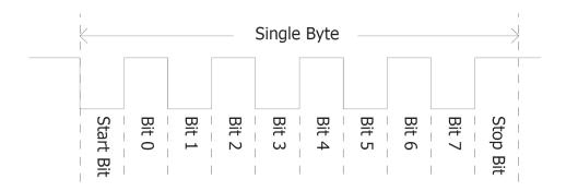
uLCD-90D Series Serial Ports - TTL Level
