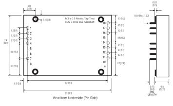
ALL DIMENSIONS IN INCHES (mm) All pins are in true position within .010 DIA. @ M.M.C. Tolerance (inches) XX  $= \pm 0.02$ .XXX ± 0.005 Heatsink adds 0.74" to height of unit.
