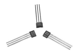
The SS490 Series MRL (Miniature Ratiometric Linear) sensors are small, versatile linear Hall effect devices which are operated by the magnetic field from a permanent magnet or an electromagnet. The ratiometric output voltage is set by the supply voltage and varies in proportion to the strength of the magnetic field.
