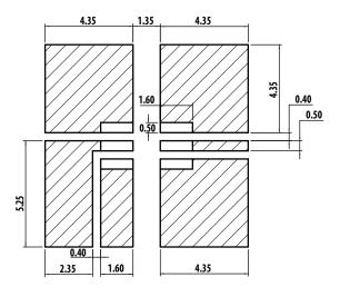
Figure 12: Carrier Tape Dimension
