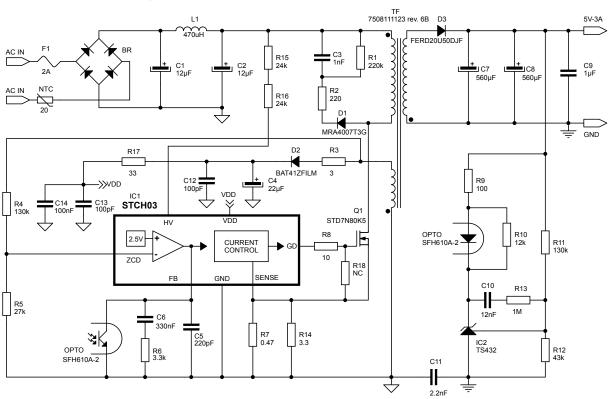
Figure 2. STEVAL-SMACH15V1 evaluation board schematic
