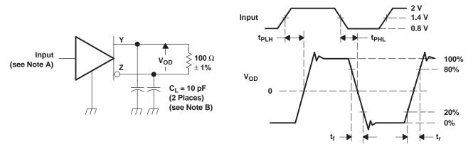
NOTES: A. All input pulses are supplied by a generator having the following characteristics:  $t_r$  or  $t_f \le 1$  ns, pulse repetition rate (PRR) = 50 Mpps, pulse width = 10 ± 0.2 ns.
