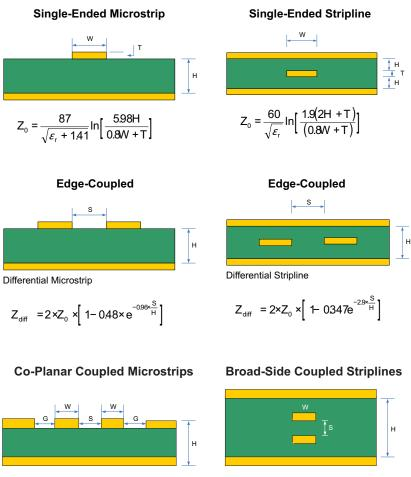
Figure 12. Controlled-Impedance Transmission Lines
