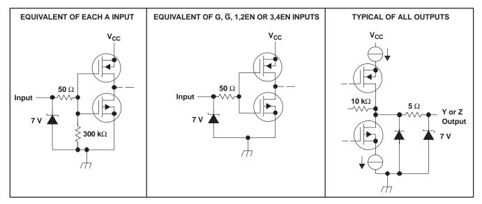
Figure 8. Equivalent Input and Output Schematic Diagrams
