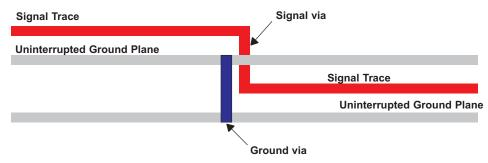
Figure 22. Ground Via Location (Side View)
