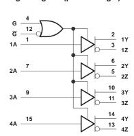
'LVDS31 logic diagram (positive logic)
