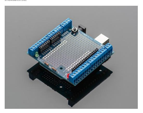
The shield even comes with stacking headers, (https://adafru.it/alH) which let you plug *another* shield on top! As shown here, a data logging shield is stacked onto the proto-screwshield.
