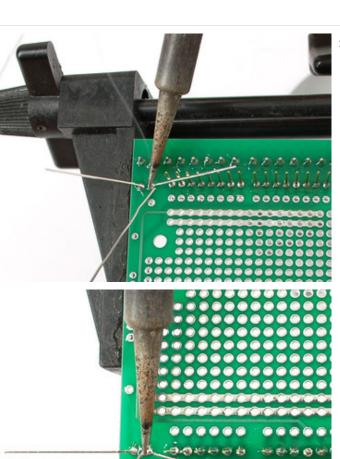
Solder both LEDs in place.
