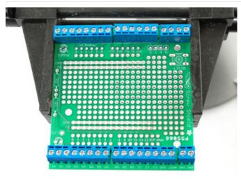
Place the remaining terminal blocks, checking again that they face the right direction!
