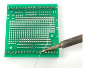
You can also just put the PCB with terminal blocks upside down on a table, which will keep the blocks in place while soldering.
