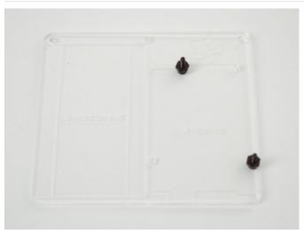
There are four mounting holes for various Arduinos. Unfortunately, each Arduino revision has slightly different 'preferred' mounting holes. Here we show what we consider the preferred holes for the Uno R3 which is likely what you have. Place the screws into the plate from the bottom of the plate so they stick up. Screw on two hex nuts to keep them in place
