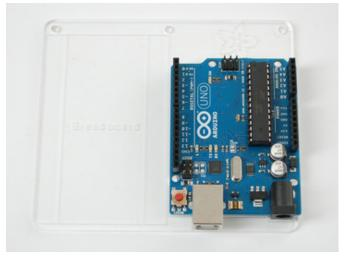
There are outlines showing how the Arduino and breadboard go on, make sure the print is right way up or it'll be confusing!
