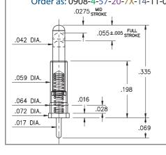
Standard Tolerances: Lengths: ± .006 Diameters: ± .002 Angles: ± 2°
