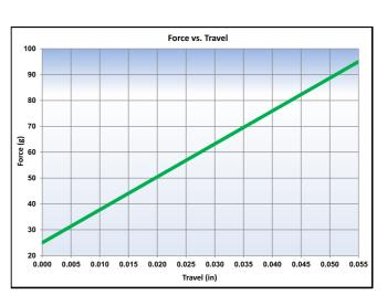
Stroke & force values are measured using spring pins with an internal construction per the design specification. Individual spring pin performance may vary from these values based on design differences.
