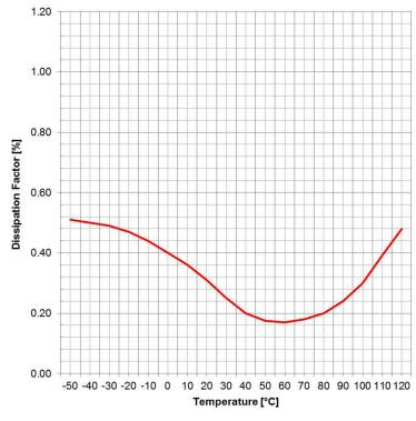
Test Equipment: E4991A or equivalent
