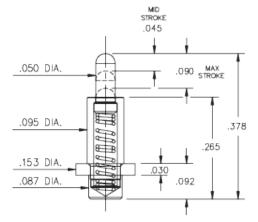
0851-0-15-20-82-14-11-0 Power Spring Pin Solder Mount in .090 min. mounting hole
