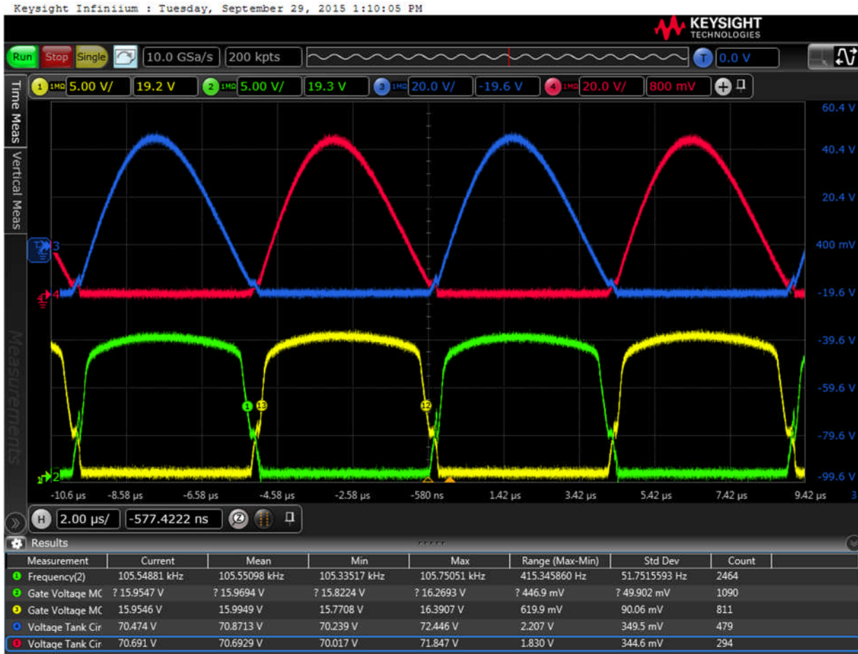
Figure 3: The voltages at the transmitter coil are shown in blue and red. The gate voltages are yellow and green (These measured voltage curves are referenced to the circuit ground GND; V_{in} = 20\text{ V} ; P_{out} = 100\text{ W} ; optimized gate drive, see application examples)
