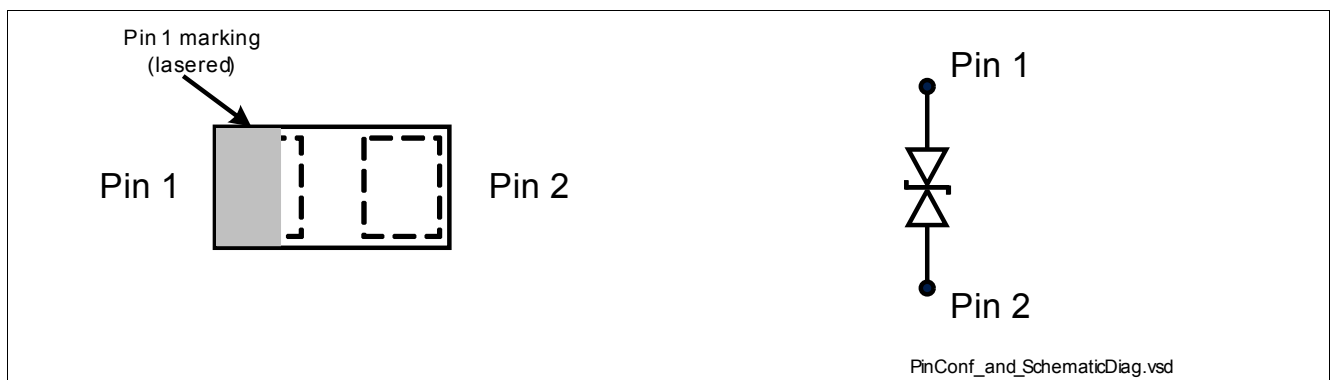
Figure 1-1 Pin Configuration and Schematic Diagram
