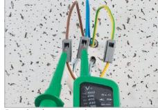
Testing through separate test slot.
