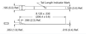
The 600-057 Micro Band is precision constructed of 300 Series SST/Passivate I.A.W AMS 2700, and designed for use with the 600-061 Hand Banding Tool or the 600-068 Pneumatic Banding Tool. Double-wrapped bands will accommodate diameters up to approximately .88 inches (22.4). Bands may be ordered flat (600-057), or precoiled (600-057-1). Bands come bagged and tagged in quantities from 1 to 100.
