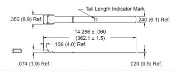
The 600-052 Standard Band is precision constructed of 300 Series SST/Passivate I.A.W AMS 2700 and designed for use with the 600-058 Hand Banding Tool or the 600-067 Pneumatic Banding Tool. Double-wrapped bands will accommodate diameters up to approximately 1.8 inches (45.7). Bands may be ordered flat (600-052) or precoiled (600-052-1). Bands come bagged and tagged in quantities from 1 to 100.
