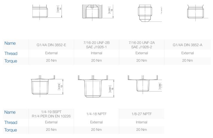
Note: Recommended torque may varify according to material and specific application.
