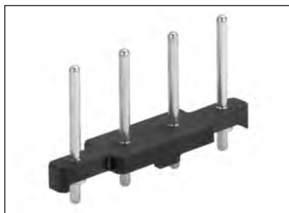
4-contact male header for THR-soldering; grid 5.75 mm
