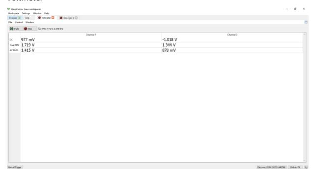
The Analog Discovery Studio's analog input pins can be used with WaveForms' Voltmeter instrument to act as a simple voltmeter. DC voltages, AC RMS voltages, and True RMS voltages can be viewed for each of the two Scope channels.
