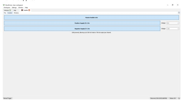
The Analog Discovery Studio has a variety of different power supply rails that are can be used to power circuits under test. The V+ and V- rails are variable, while the rest are fixed. The fixed rails are summarized in the table below:
