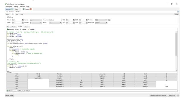
The Analog Discovery Studio can be used with WaveForms' "Protocol" instrument to work with common communications protocols. UART, SPI, I2C, and CAN transactions can be received, transmitted, and/or spied upon by the Analog Discovery Studio using any of the 16 digital input/output channels at a sample rate of 100 MS/s.
