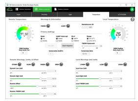
ALERT/THERM2 control in the Warnings & Information section. The Conversion Rate adjust the period of time between ADC conversions of the temperature sensor; subsequently, changing the period of the update to both the Remote and Local Temperature gauges.
