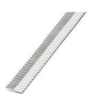
Taped ferrules,  $0.5~\text{mm}^2$ , sleeve length 8 mm, with plastic collar, according to DIN 46228-4, white, for processing with the CRIMPFOX 4 IN 1, 10 strips each with 50 sleeves per strip.
