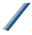
Taped ferrules,  $2.5~\text{mm}^2$ , sleeve length 8 mm, with plastic collar, according to DIN 46228-4, blue, for processing with the CRIMPFOX 4 IN 1, 10 strips each with 40 sleeves per strip.
