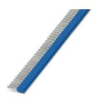
Ferrule, Dimensions according to DIN 46228-4, with color-coded plastic collars according to NF C 63-023:1994-02, for processing with the CRIMPFOX 4 in 1, sleeve length: 8 mm, color: blue, number of strips: 10, number of sleeves per strip: 50
