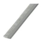
Ferrule, Dimensions according to DIN 46228-4, with color-coded plastic collars according to NF C 63-023:1994-02, for processing with the CRIMPFOX 4 in 1, sleeve length: 8 mm, color: gray, number of strips: 10, number of sleeves per strip: 40
