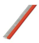
Taped ferrules, 1.0 mm<sup>2</sup>, sleeve length 8 mm, with plastic collar, according to DIN 46228-4, red, for processing with the CRIMPFOX 4 IN 1, 10 strips each with 50 sleeves per strip.
