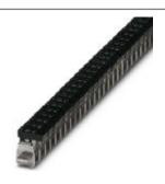
Connection terminal block, connection method: Screw connection, load current: 76 A, cross section: 1.5 mm² - 16 mm², width: 9.8 mm, color: black
